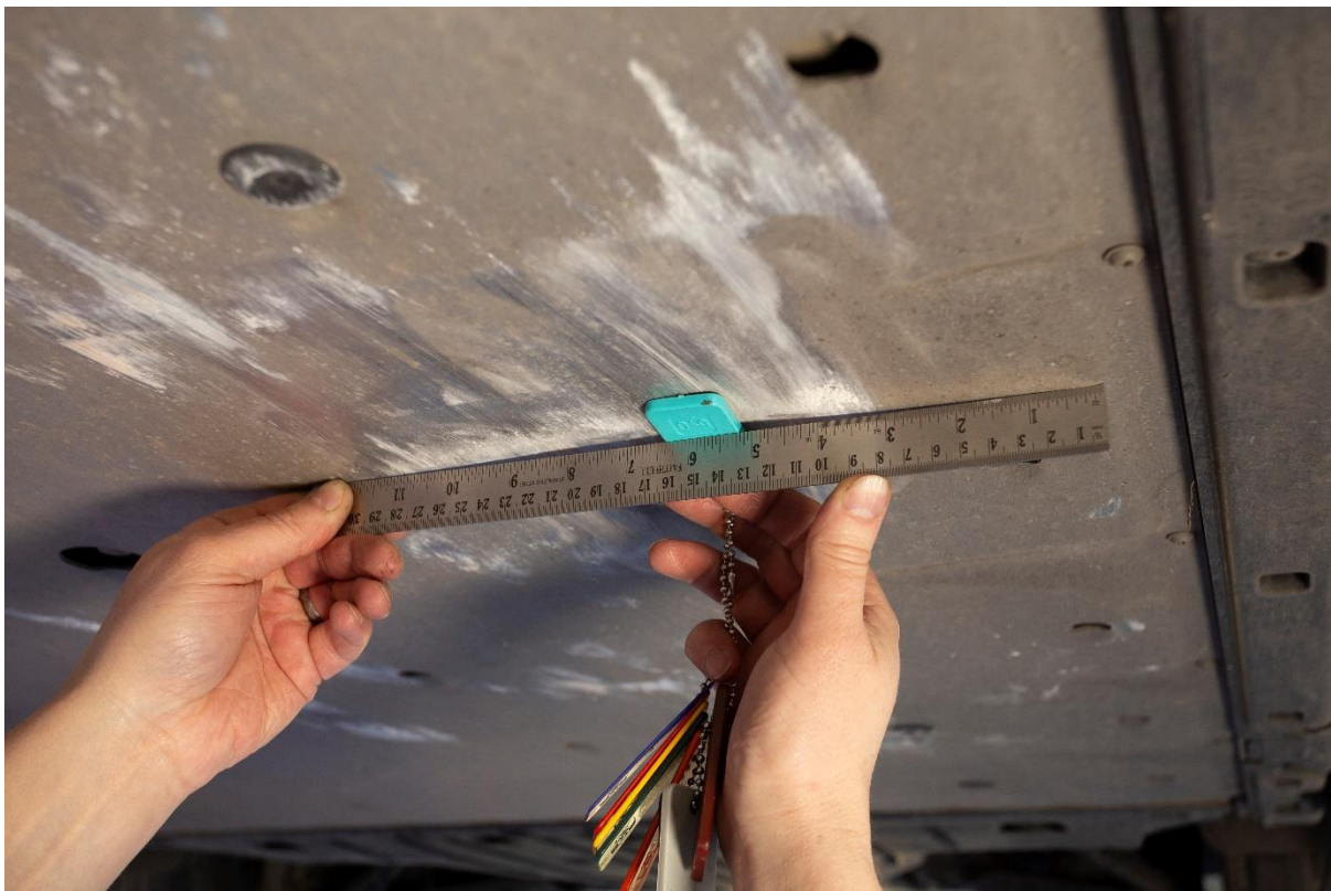
Figure 20 – Volkswagen ID4 battery underside with an abrasion 5mm in depth.
