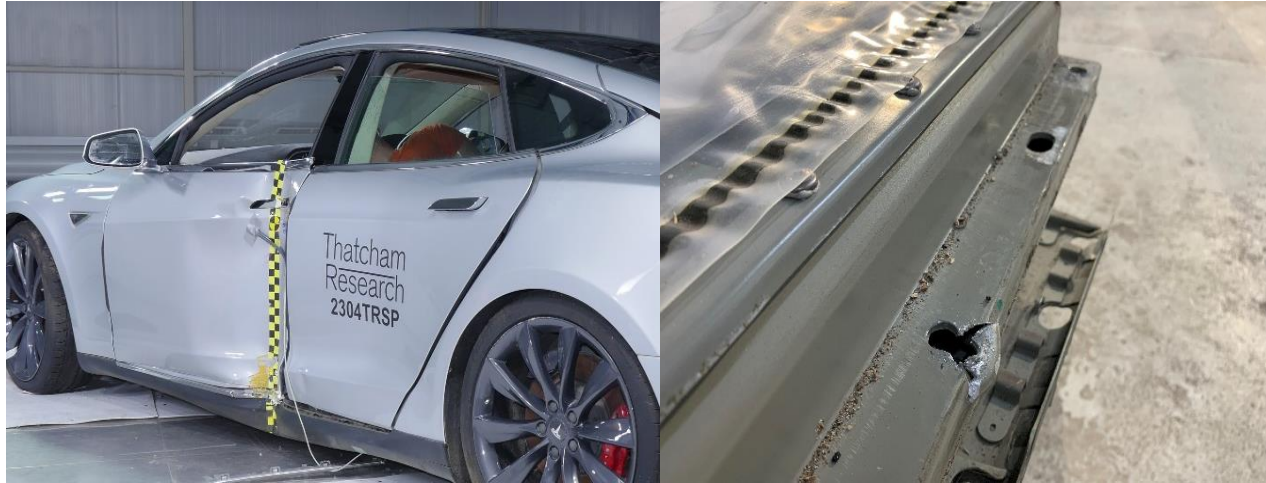
Figure 10 – Thatcham Research low severity crash test (Left) with resulting damage to battery casing (Right) .
