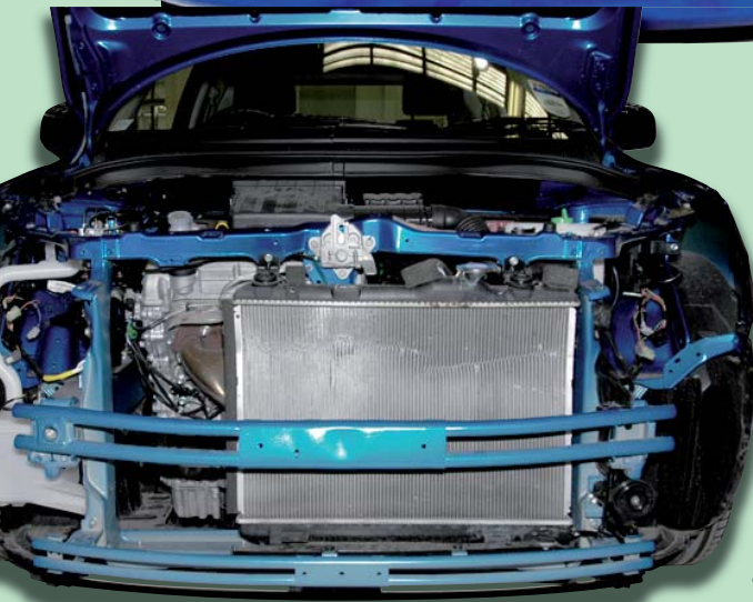
Suzuki Swift front £2,300 : Top picture: with bumper cover in place. Bottom picture: cover removed to show bumper beam
