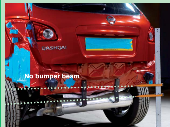
Nissan Qashqai: Poor bumper system with no bumper beam at all
