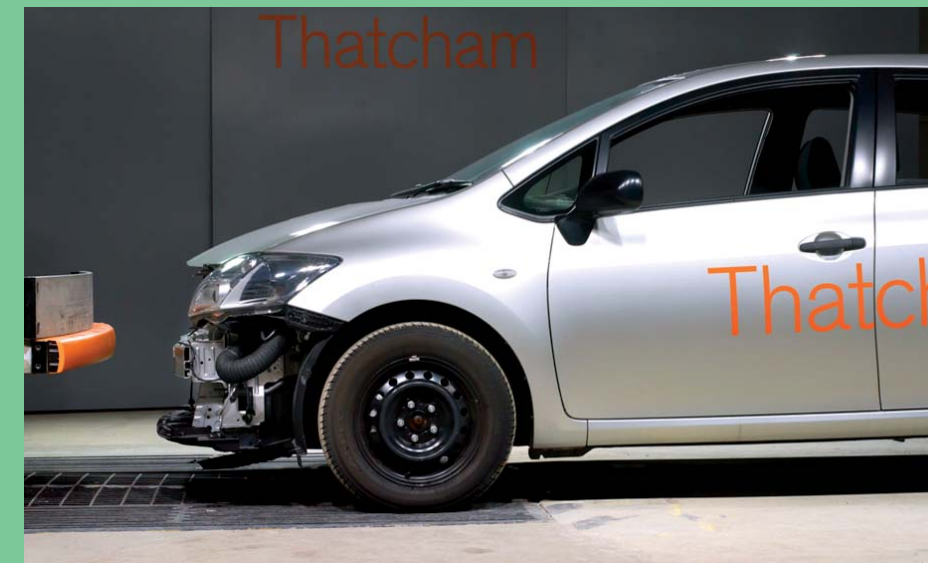
Front bumper test with bumper cover removed to show beam alignment
