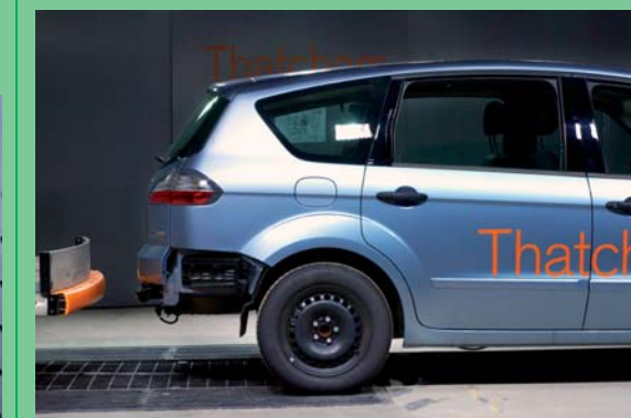
Rear bumper test with bumper cover removed to show beam alignment
